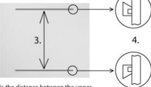
The measurement you've chosen is the distance <u>between</u> the upper and lower mounting rails. (See fig. 3)
